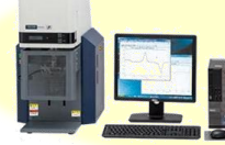
Linear expansion measurement
