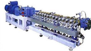
Material development equipment (2-axis extruder)
