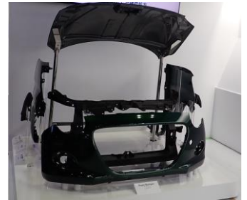
A concept that makes extensive use of plant-derived resins Exhibited at the Automotive Engineering Exposition 2023
